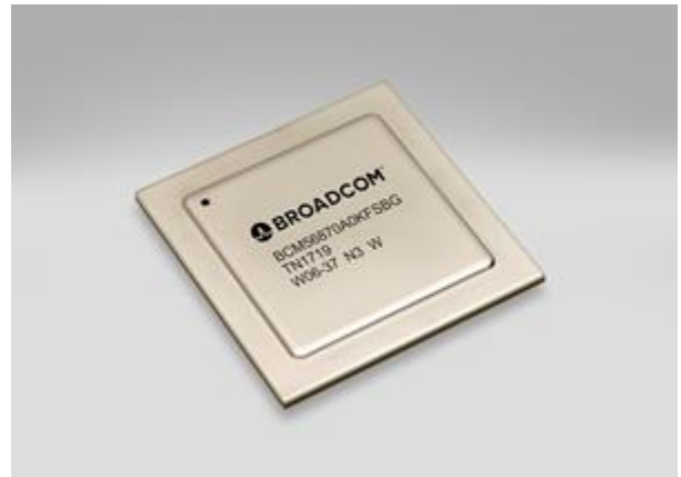
The Broadcom Trident 3 is an ethernet switch with new levels of data plane programmability
